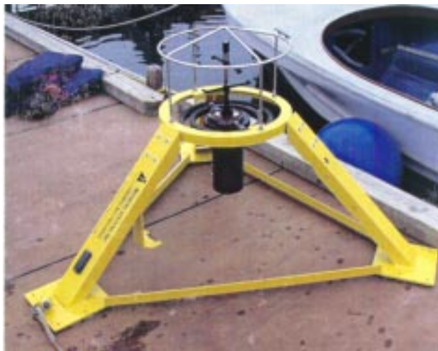
Figure 4. The 3D Wave Height and Direction Current Meter by Falmouth Scientific Instruments
